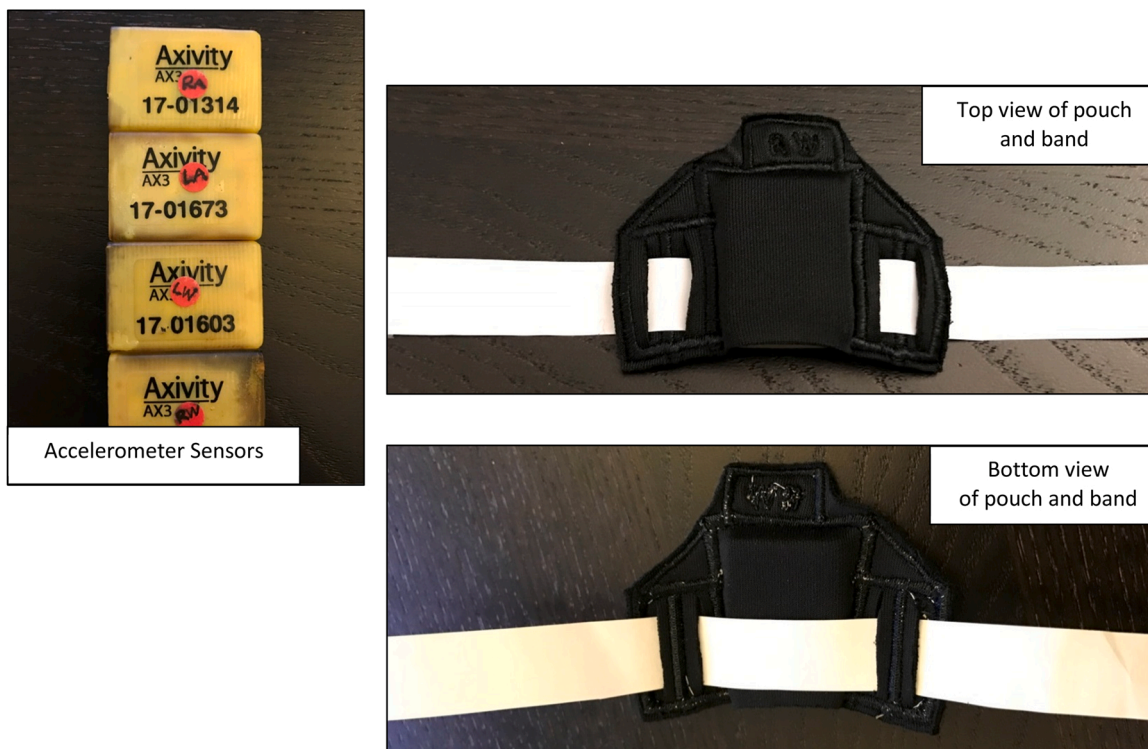
Fig. 2. Accelerometer sensors, pouches, and wrist/ankle bands.
